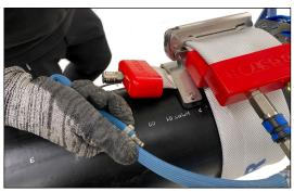
Now connect the short coupling hose to the longitudinal pressure rail.
