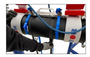
Connect the welding cables, sensor wires and return air hose from the reduction box to the front of the WeldMaster/WeldMaster Light.
