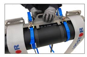
Release the check valve in the three pressure bands with a blunt tool.
