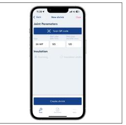
If the QR-code is damaged or unavailable, manual choices can be made by pressing the input fields. When inserting the information manually, the production order ID linked to the casing joint cannot be saved in our database.
