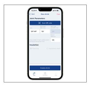
Select insulation The insulation type is preselected and greyed out, if there is only one type available for the casing joint selected. However, some casing joints can be installed with either insulation shells or
