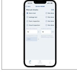
If the measurement is not approved, the input field will display a red outline and the text: "Not approved according to LOGSTOR accept criteria".
