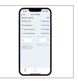
Foam inspection Press "Foam inspection", if there was visible foam at the venting plugs (Insulation type: Foaming) or if the insulation shells have been installed tightly between the casing pipes (Insulation type: Insulation shells).
