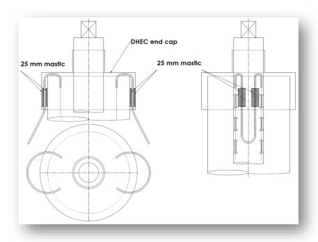
This will thus be the standard solution on pre-insulated stop valves without a service valve and on pre-insulated valves with 1 or 2 service valves.
