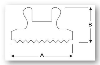
Wall entry sleeve dimension 110 – 180 mm A = 40 mm and B = 22 mm
