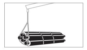
Place 2 straps around the middle of the pipe bundle approx. 4 m from each pipe end.
