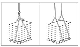
When unloading pallets place the straps under the pallet in one of the following two ways.
