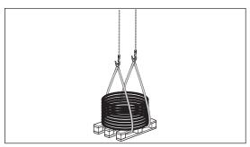
Place the straps under the pallet without the straps getting in contact with the coil.
