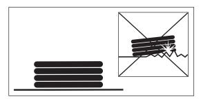
Always place coils on an even surface, so that they have the maximum supporting surface. The substratum must not contain stones that might damage the jacket.
