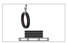
If only the top coil is to be unloaded from a pallet, a flat strap is placed around the the coil as illustrated.
