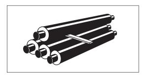
Place a wooden sleeper between the pipes and lower the pipes again.
