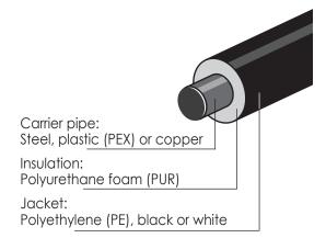
The pipe dimensions are indicated as follows: 76,1 mm / 140 mm
