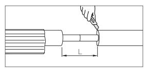
2. Cut away expanded insulation from the pipe ends (L = max. 300 mm).
