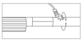
8. Activate the jacket pipes at least 150 mm from both sides of the pipe ends until the surface has a matt, silky look.
