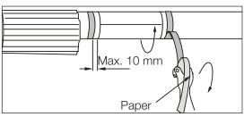
Remove the paper from both mastic strips. Place the adhesive side face down on the jacket pipe and away from the insulation shells. Place the mastic strips max. 10 mm from the jacket pipe end.
