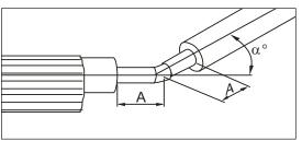
3. The shrink sleeve is applicable at angles of 0°-15° ( $\alpha$ °). A = max. 150 mm.
