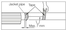
7. To cover gaps use linen tape or PVC free tape, overlapping the jacket by max. 7 mm.
