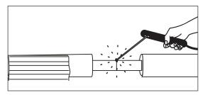
1. Place the shrink sleeve on the pipes. Weld the steel pipes. Pressure test.
