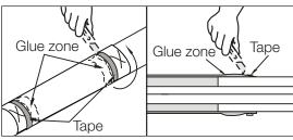
12. Wind the tape around the sleeve, where the glue zone is faintly marked. Use a very sharp knife to cut along the edge of the tape while the workpiece is still hand-warm.
