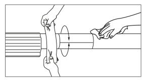
Clean the jacket with tissue. Activate the jacket pipes with EMERY CLOTH at least 80 mm from both jacket ends. Use EMERY CLOTH to remove sharp edges or burrs on the jacket pipes.
