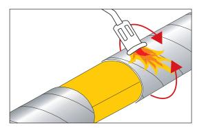
5. Centre the shrink film over the joint around the pipe.
