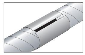
8. Place a steel strap or similar approx. 50 mm from each end and tighten it. This is done at the same time at both ends.
