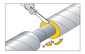
2. Shorten the insulation shells, so they fit tightly between the Spiro pipes.
