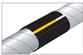
Heat the film from the middle towards both sides, so the mastic becomes visible at all edges and the entire shrink effect has been utilised.
