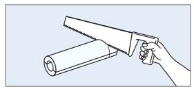
4. Shorten the mineral wool shells to make them fit tightly between the jacket pipes.
