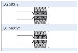
16. Mount the welding elements with nails as shown above and with a nail each 250 mm around the jacket pipes.
