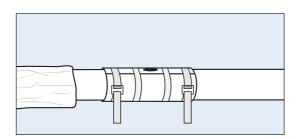
6. Centre the aluminium foil over the joint. Tighten the straps. Wind filament tape round the foil on both sides of the hole.
