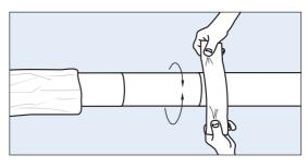
9. Wait minimum 30 minutes for degassing. Remove the aluminium foil. Activate the jacket pipes with abrasive cloth grain size 80 at least 150 mm from both jacket ends.
