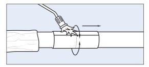
12. Heat the whole film from the centre outwards, ensuring that the mastic becomes visible at all edges and that the shrink film is tightly fitted.
