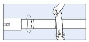
14. Pull the sleeve away on the cleaned pipe end. Thoroughly activate the jacket pipes with abrasive cloth, grain size 36-40, exactly touching the marking.
