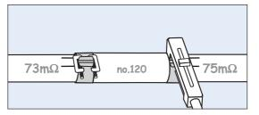
19. Mount clamps 5-10 mm over the sleeve ends. Press the clamps until the jacket pipe starts to deform (max. 0.1 mm). Keep the clamps tightly positioned by using a clamping tool.
