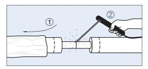
1. Place the shrink sleeve with packing on one of the pipes, before the carrier pipes are joined.
