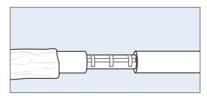
5. Fit the mineral wool shells tightly between the jacket pipes, using canvas tape if required.
