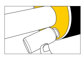
Hammer the coupling approx. 25-30 mm into the foam.
