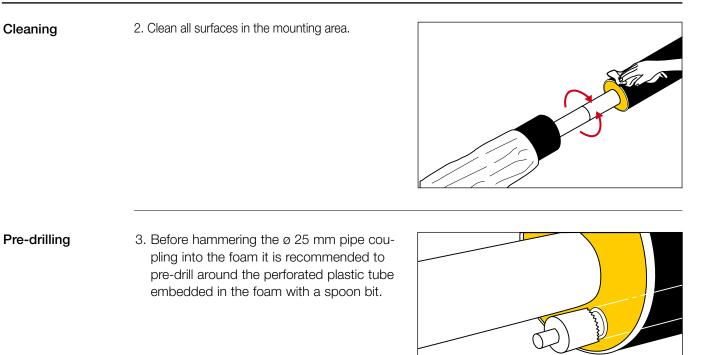
Installing the pipe coupling
