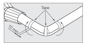
4. Fasten the insulation shells with tape. The tape overlap on the jacket is max. 10 mm.
