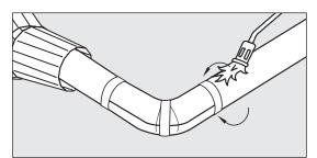
6. Activate the jacket pipes at least 150 mm from both jacket ends until the surface has a matt, silky look.
