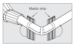
7. Pull the paper off the adhesive side of the mastic strip. Place the adhesive side face down on the jacket pipe furthest from the insulation shells.
