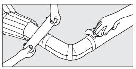
Clean the jacket with tissue. Activate the jacket pipes with ABRASIVE CLOTH at least 80 mm from both jacket ends. Use ABRA-SIVE CLOTH to remove sharp edges orr burrs on the jacket pipes.
