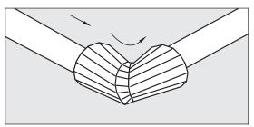
8. Remove the packing from the shrink sleeve. Check that it is CLEAN and DRY, inside and out. Centre the shrink sleeve on the elbow.
