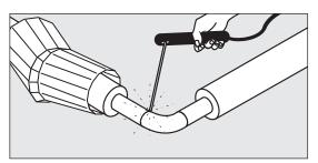
2. Weld the steel pipes. Pressure test.
