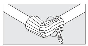
9. Start shrinking at the top of the shrink sleeve 5-8 cm from the end. During shrinking it is possible to adjust the position of the shrink sleeve.
