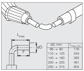
Place the two pipe ends at the correct angle. Pull the shrink sleeve onto the pipe (F = max. 150 mm).
