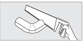
3. Cut the insulation shells to make them fit over the steel pipes.
