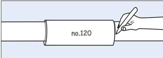
13. Remove the packing from the shrink sleeve. Do not use cutting tools. Leave the packing on the pipeline. Check that the sleeve is CLEAN and DRY, inside and out. Centre the sleeve over the jointing area. Mark the placing of the sleeve on the jacket pipes. Write the sleeve number on the sleeve. Fill in the documentation form.
