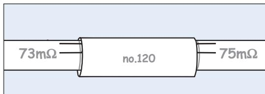
17. Place the sleeve between the marks. Write the joint number and resistance values for the welding element on the sleeve/jacket pipes and in the documentation form.
