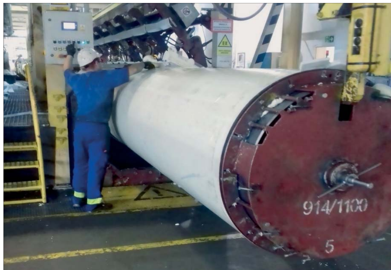
Figure 3. During the production of the Opti pipe, the foam is visually checked along its full length
