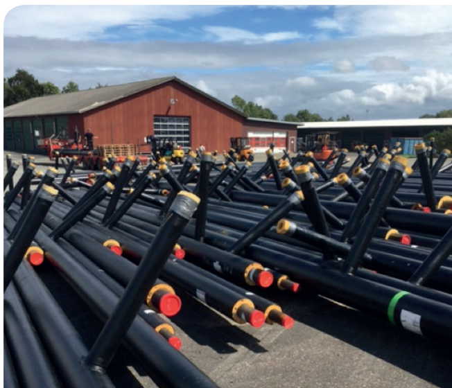
Fig. 8 and 9 - Standpipes made indoor. In the indoor factory, straight pipelines are manufactured with standpipes, designed so they match the exact position of the solar panels.
