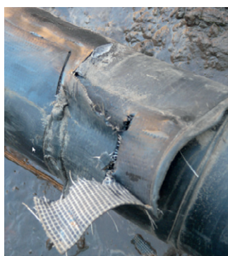
Fig. 4 - Shrink wrap peeled off due to the large number of movements.
