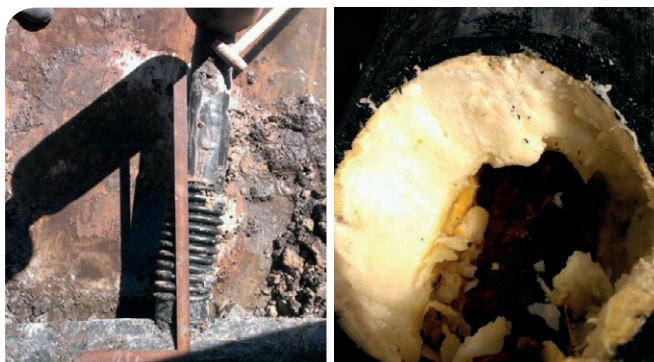
Fig. 1 - Branch, damaged by large movements.
