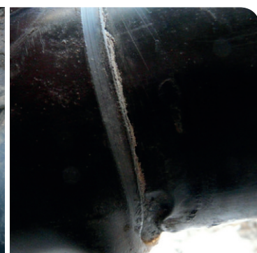
Fig. 5 - Dislocated casing joint due to the large number of movements.
