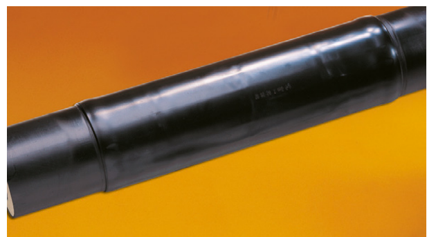
Correctly installed: the expansion marks have disappeared and the shrinkable ends are flat and smooth
